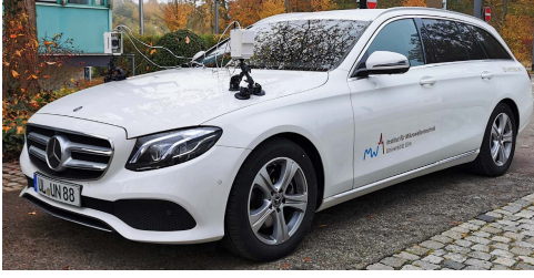
Fig. 2. Experimental system setup with two side-look radar sensors on a car.
