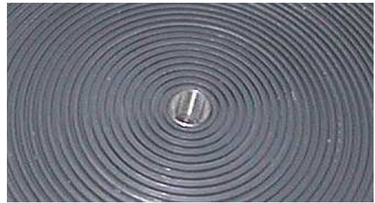
Fig. 6: Surface matching of the lens using milled groves.
