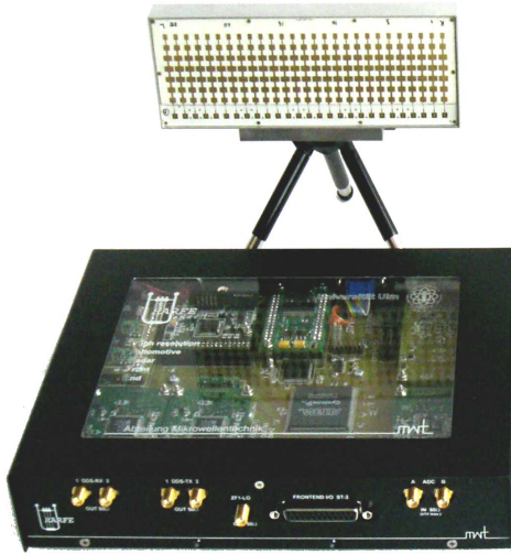
Fig. 2. Photograph of the HARFE Experimental System with the front-end (top) and the radar electronics (bottom).
