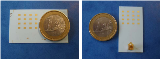
Fig. 5 Photographs of the realised antenna with coplanar interface (left) and with mini-SMP connector (right)
