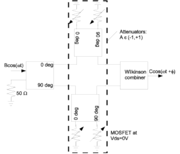
Figure 23. Schematic of the Vector Modulator (VM) with tunable RfMOS terminations.
