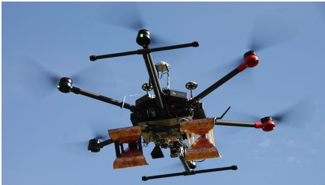
Fig. 6. Photo of the measurement system. It consists of a DJI Matrice 600 Pro, a DJI D-RTK GNSS mounted on the top of the UAV, and the GPSAR sensor module mounted below the UAV.
