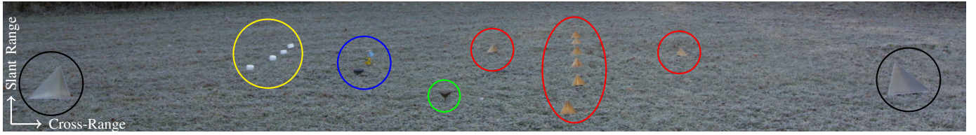
Fig. 5. Photo of the measurement setup from the perspective of the radar. The setup consists of 8 reflectors with an RCS \sigma_1 = -12.2 dBsm (red), 1 reflector with an RCS \sigma_2 = -15.3 dBsm pointing upwards (green), 2 corner reflectors with an RCS \sigma_3 = 3.7 dBsm (black), 3 metal cans (blue), and 4 plastic boxes (yellow). All targets have been placed on the ground.
