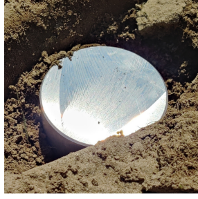
(b) Aluminum cylinder, diameter 8 cm, height 4 cm (CYL).
