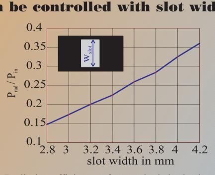
Radiation efficiency of a matched single slot pair over slot width ( $\varepsilon_r$ =2.33, h=0.79 mm,  $w_{\text{metal}} = w_{\text{slot}} + 200 \mu \text{m}, w_{\text{inner}} = 0.5 \text{ mm}, l_{\text{slot}} = 3 \text{ mm})$
