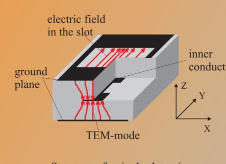
Structure of a single slot pair
