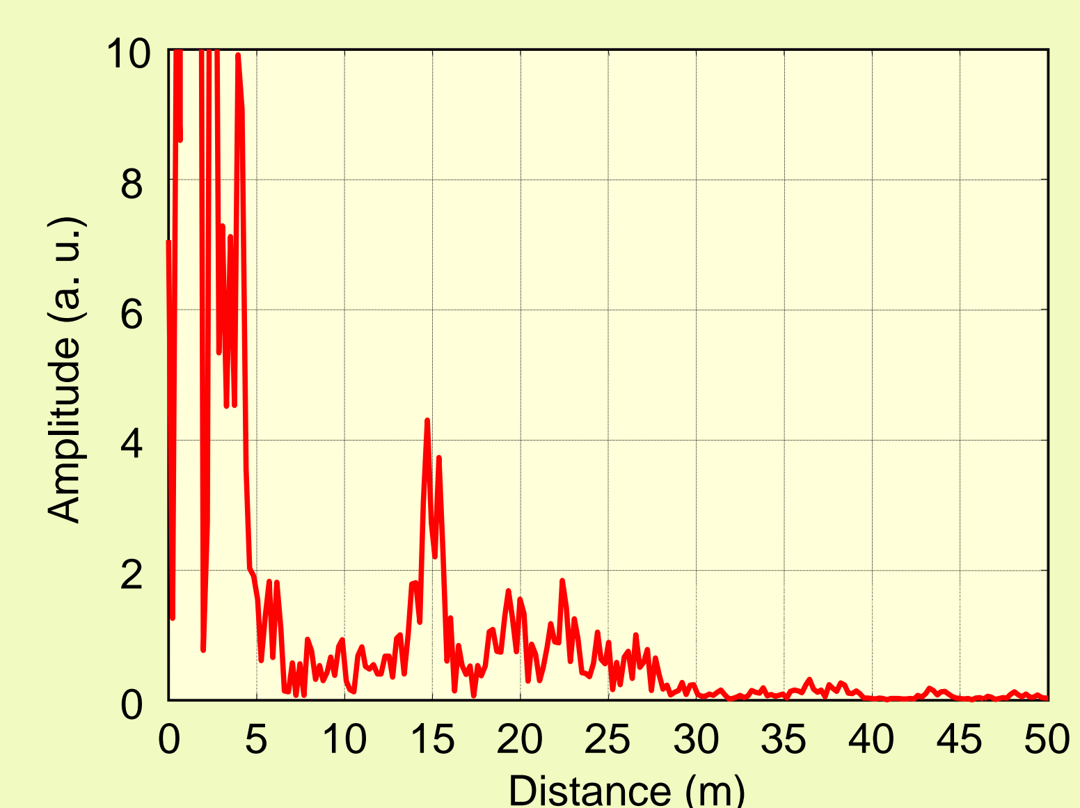
FFT of a reflector of 1m² radar cross section at a distance of 15 m (no range filtering)
