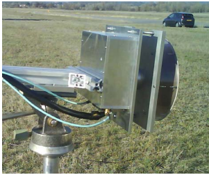
Fig. 2: Sensor with planar folded reflectarray antenna.
