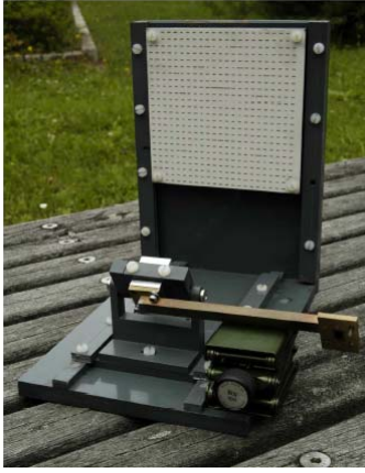
Fig. 12 Offset feed antenna for investigation of the structures in farfield measurements.
