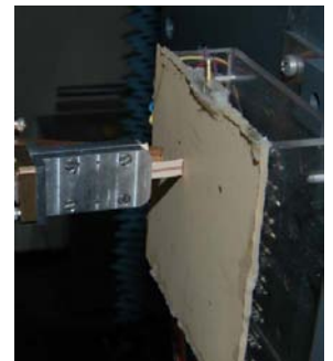
Fig. 1 Near-field measurement setup for reflectarray characterization with a liquid crystal reflectarray as DUT.
