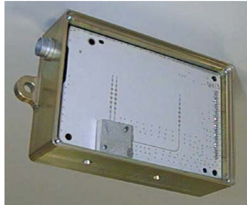
Fig. 3. 79 GHz UWB SRR demonstrator based on SiGe technology (source: Continental AG)
