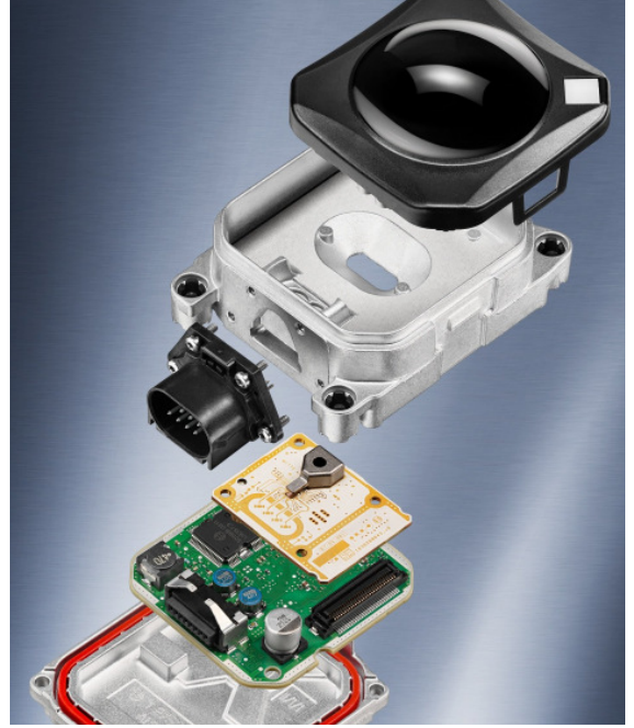
Fig. 2 Exploded view on the LRR3 automotive radar of Bosch [25] (photography by Bosch).
