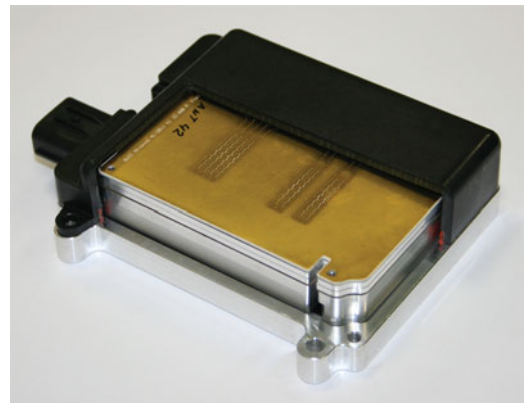
Fig. 11. RoCC sensor package, cut open to show the interior.
