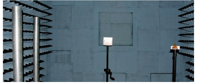
Fig. 8. Measurement setup with two metal tubes at radial distances of 2.45 m and 3.78 m on the left-hand side, a metal plate at the center with a distance of 4.96 m and a corner reflector at a radial distance of 3.09 m on the right-hand side as targets.
