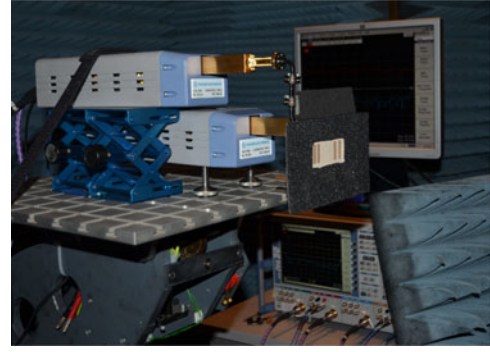
Fig. 5. Measurement setup for the estimation of the two-way pattern.
