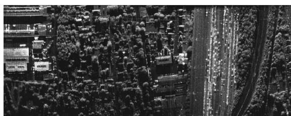
Figure 3. A UAV SAR image of urban terrain taken with a MIRANDA radar, offering 1-GHz bandwidth. (Used with permission from [13].)
