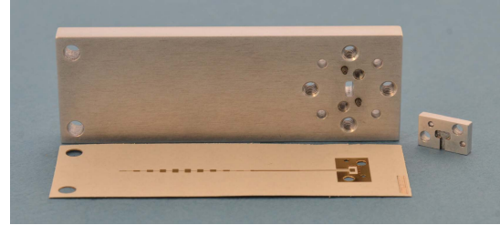
Fig. 4. Fabricated series-fed microstrip patch array on RO3003 substrate from Rogers Corporation [19] with 127 \mu\text{m} thickness.
