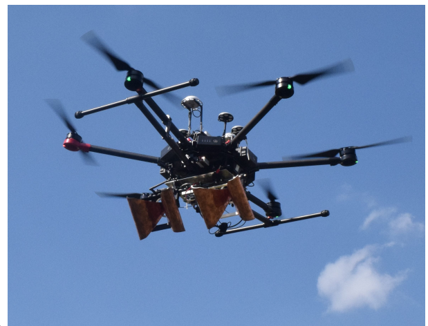
Fig. 1: Carrier platform DJI M600 Pro equipped with two light-weight broadband antennas.
