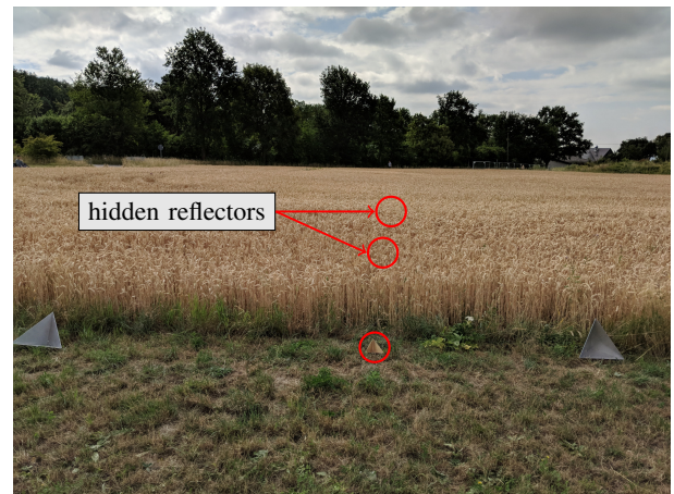
Fig. 8: Measurement field with two 30 dBsm corner reflectors and three -13 dBsm corner reflectors.
