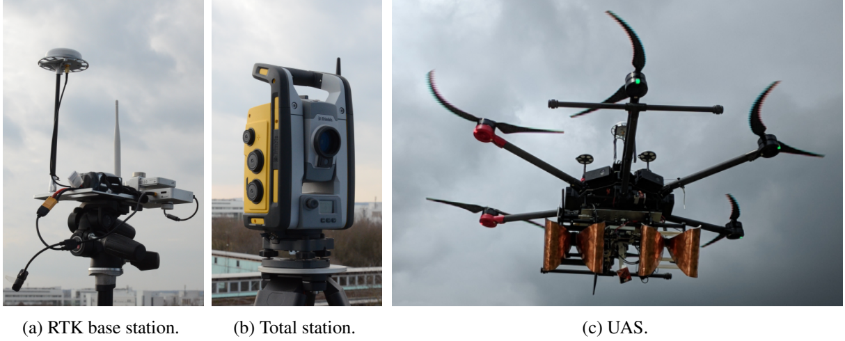
Figure 1: Measuring system consisting of an RTK base station, a total station, and the UAS. The UAS is equipped with an RTK GNSS rover station, a 360°-prism, a single-board computer for data storage, and the bistatic FMCW SAR.
